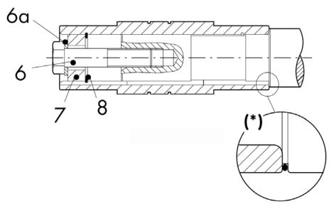
(\*) An O-ring is recommended to provide increased protection against moisture.
