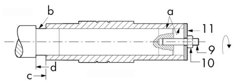
To prevent the shaft slipping, the screws must be tightened to the torque value specified in the table below in order to be able to transmit the output torque indicated on the type identification plate.
